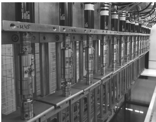
Fig. 2 Test rig with individually controlled specimen holders and motors
